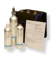
Custom and standard gas mixtures and pure gases are available from Air Products in a range of lightweight, aluminium non-refillable cylinders, ideal for applications where portability is essential. Gas mixtures are blended gravimetrically (generally according to the principals of ISO6142) and when combined with our advanced cylinder preparation techniques ensure mixture accuracy, optimum stability and maximum shelf life.
